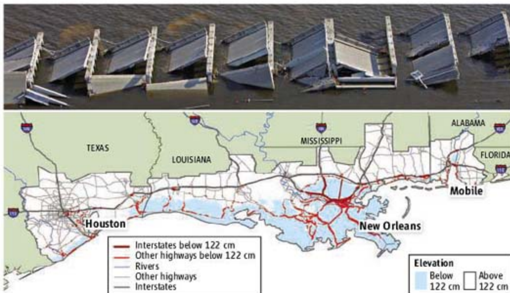
Road hazards. New study (above) shows what a 122-cm rise in sea level would do to the Gulf Coast's major roads, already vulnerable to major storms such as Hurricane Katrina in 2005 (top).
